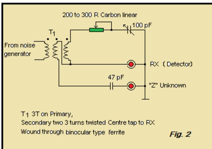
Photo 2. Noise Bridge for series equivalent impedances.
