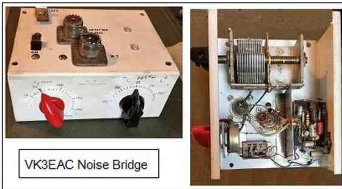
Photo 1. Noise Bridge for parallel equivalent impedances. (See Photo 3 for connection detail)
